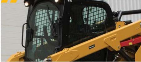
The D3 Series incorporates an industry-leading, totally enclosed, one-piece modular style cab, with a tilt up design for unparalleled serviceability and underside accessibility.
