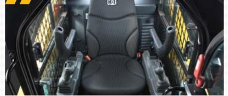
The D3 Series offers an optional, industry-first, high-back, heated, air ride seat with seat-mounted controls.
