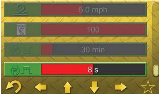
The “Reversing Fan Duration” is the duration of each reverse cycle in the automatic mode. The fan will automatically return to the forward air flow direction after each reverse cycle.
