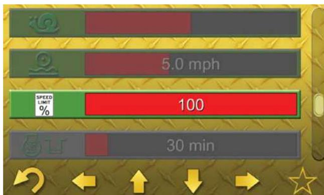
The “Machine Speed Limit Adjustment” allows the maximum travel speed to be limited. The adjustment can be made in 1% increments from 20% to 100% of the machine’s maximum travel speed.
