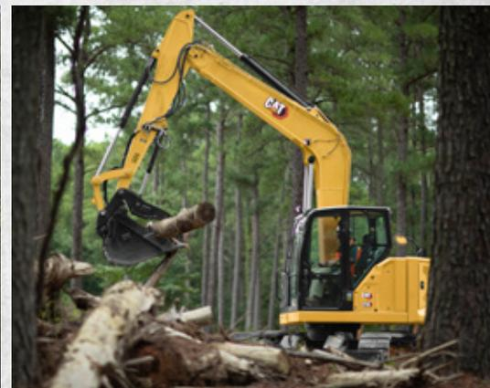
» **Standard tail swing** provides optimal leverage to create an incredibly stable working platform during lifting and digging.
