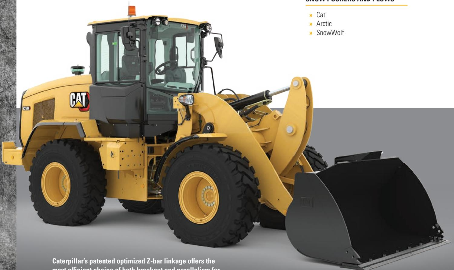
Caterpillar's patented optimized Z-bar linkage offers the most efficient choice of both breakout and parallelism for whatever your job requires. Available in both standard and high lift configurations.
