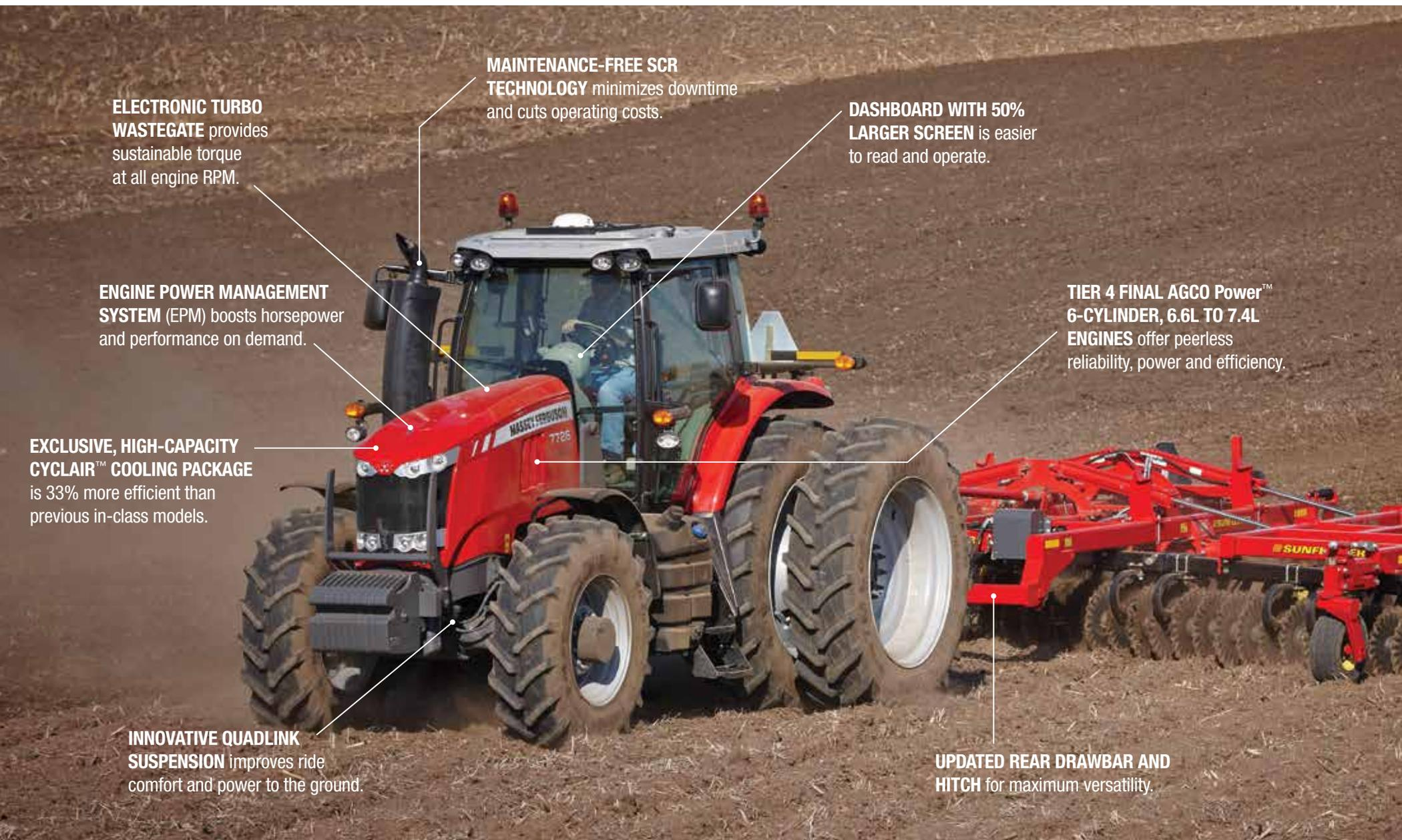
**ELECTRONIC TURBO WASTEGATE** provides sustainable torque at all engine RPM.
