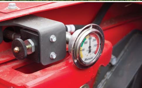
Hydraulic conditioning roll tension on the 1393 & 1316S. This is the first pull-type design to have this system.
