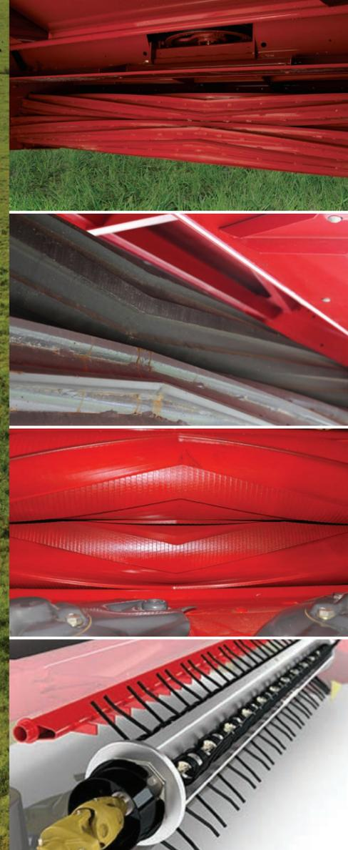
**STEEL-ON-STEEL ROLLS** Designed to meet the needs of custom and commercial operators, steel-on-steel rolls feature a herringbone pattern that provides long-lasting durability while evenly distributing crop material across the full width of the rolls. They're also the best option for alfalfa, since they crimp the stems, for faster drying while maintaining leaf quality.
