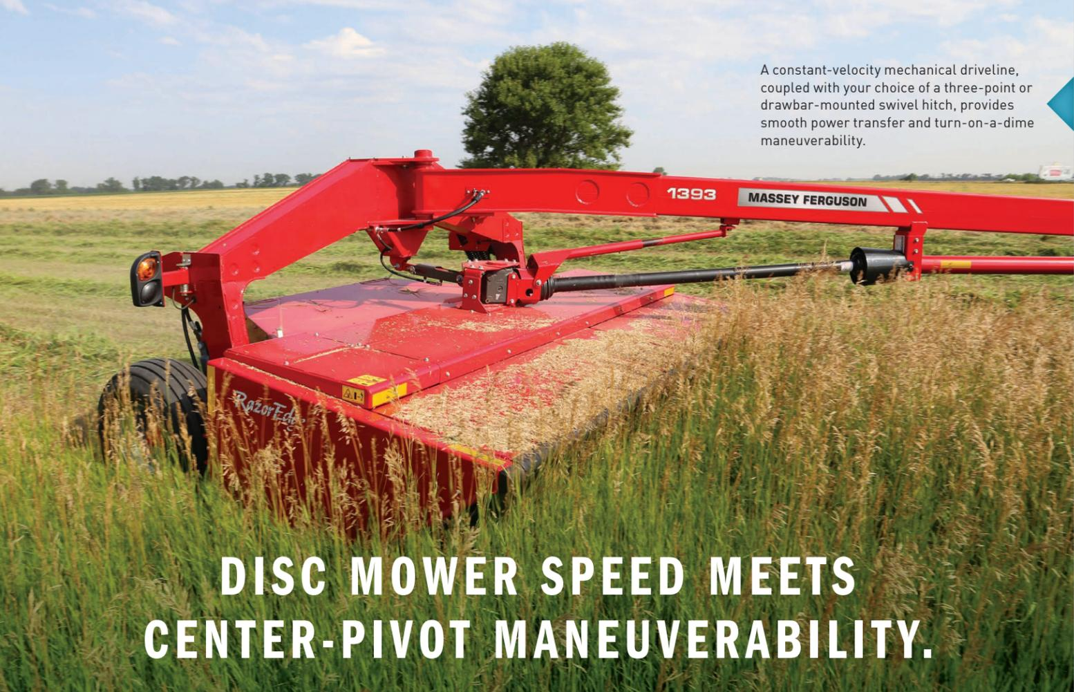
A constant-velocity mechanical driveline, coupled with your choice of a three-point or drawbar-mounted swivel hitch, provides smooth power transfer and turn-on-a-dime maneuverability.
