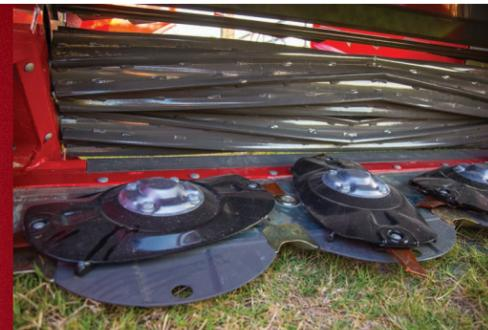
**THE RAZOREDGE CUTTER BAR'S DESIGN** allows each gear assembly and adjacent idler gear to be individually removed without disassembly of the cutter bar. The spur gear design also provides a thinner profile, allowing closer cutting with less scalping.
