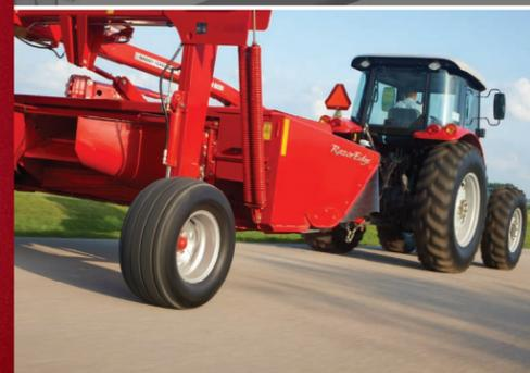
**THE HIGH-CLEARANCE MAINFRAME** provides an exceptional header lift height of 20 inches for better clearance over headland windrows. The added height also allows the header to be easily carried over obstacles, ditches and waterways.
