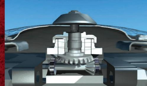
**EACH CUTTER BAR** is driven by a segmented, reversible hex drive shaft for quick disassembly and reduced operating costs. The hex drive shaft is also designed to absorb the shock of hitting an obstruction, reducing the risk of damage.
