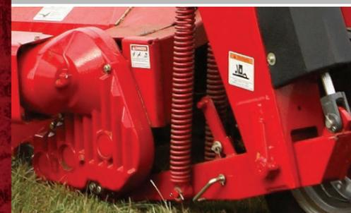
**SPRING TENSIONING** supports the cutter bar through a variety of field conditions, increasing efficiency and reducing wear.
