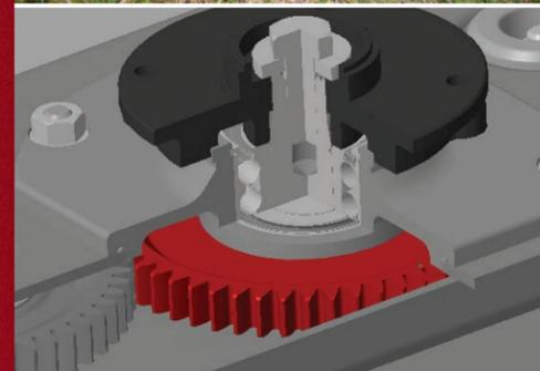
**THE INTERNAL SPUR GEARS** offer 2.5 teeth contact at all times to transfer high torque and seamless power throughout the entire cutter bar. Gears are forged in house at the AGCO Power Foundry
