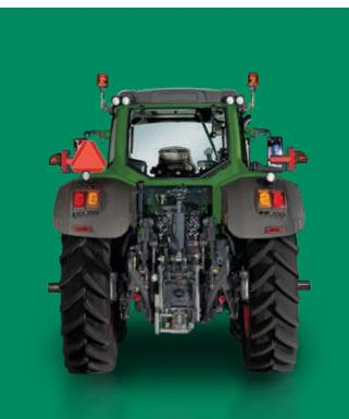
The ability to produce down-force pressure on the front (optional) and/or rear 3-point hitch is particularly valuable when operating certain types of tillage equipment — or for simply raising the tractor to install or remove dual wheels.
