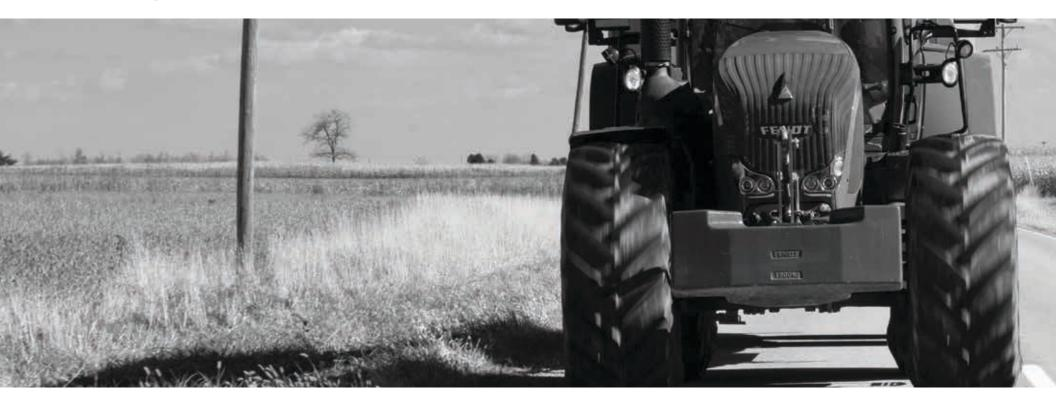
Regardless of the model or payload, the front and rear axle on each Fendt Series was designed to handle the horsepower and permissible axle loads. The adaptable drivetrain also incorporates four-wheel braking to stop those big loads, even at high transport speeds, for greater safety, optimum brake force distribution and full steering capability while stopping.
