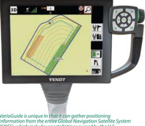
VarioGuide is unique in that it can gather positioning information from the entire Global Navigation Satellite System (GNSS), which includes constellations owned by the U.S. (WAAS), the Russian Federation (GLONASS) and the European Union (Galileo). The greater satellite availability means greater accuracy and fewer signal interruptions.
