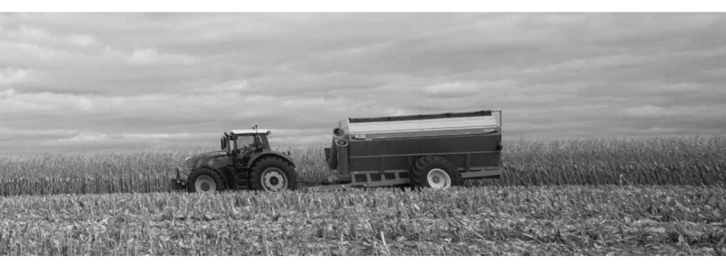
Responsive power and maximum efficency come together in every Fendt tractor, regardless of the model. While the Fendt 700 and 800 Series feature a 6.06-liter, six-cylinder Deutz diesel engine, the 900 Series boasts a tough 7.8-liter, six-cylinder Deutz diesel. Both utilize Fendt SCR (selective catalytic reduction) technology to provide up to 10 percent better fuel economy and higher torque rise (up to 43 percent) than previous models all while meeting Tier 4 Final emissions standards.
