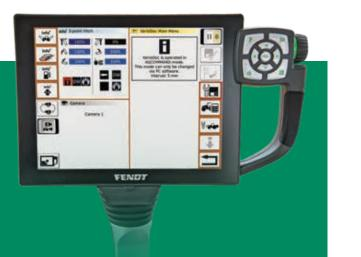
Monitor and adjust all tractor functions, including the transmission, hydraulic system, 3-point hitch, headland management system, service and diagnostics.
