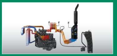
SCR (Selective Catalytic Reduction) exhaust gas after-treatment
