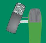
Without VarioActive 1 turn of the steering wheel = 26.6° *With VarioActive* 1 turn of the steering wheel = 43.3°
