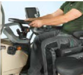
For enhanced operating comfort, the cockpit swings parallel with the steering wheel. Easy steering wheel adjustment via a separate foot pedal, hands-free for adjustment.
