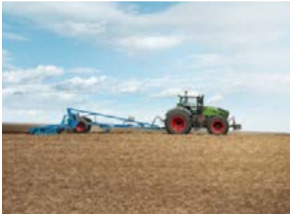
Thanks to the TMS tractor management system and the automatic maximum load control 2.0, the tractor adapts the engine speed optimally to the road speed.
