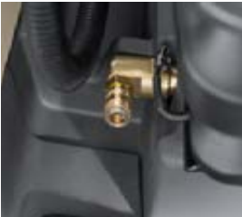
The cab is cleaned quickly: The driver seats (super comfort seat Evolution) have a practical connection for a compressed air hose, which can be used to clean the cab.
