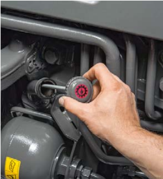
Maintenance activities, such as checking the oil level or changing the filter, a performed quickly and easily on the Fendt 1000 Vario. The engine compartment is especially easy to access thanks to the removable side panels.
