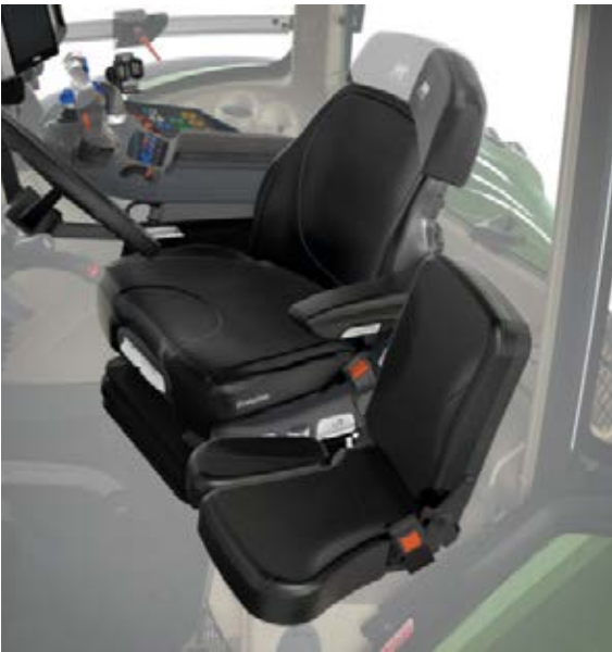
The comfort passenger seat is ergonomically formed and has additional cushioning. Folded down, it turns into a practical table with a clamp for papers.
