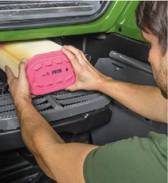
The cab filter is easily accessible in the door area and can be easily cleaned when necessary.
