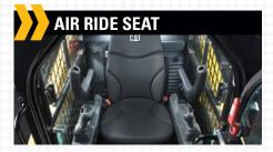
The D3 Series offers an optional, industry-first, high-back, heated, air ride seat with seat-mounted controls.
