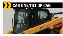
The D3 Series incorporates an industry-leading, totally enclosed, one-piece modular style cab, with a tilt up design for unparalleled serviceability and underside accessibility.
