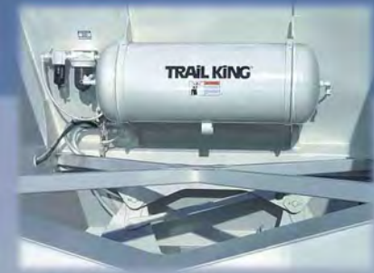
Large Air Reservoir, with air system oiler, means longer operating time and better control.
