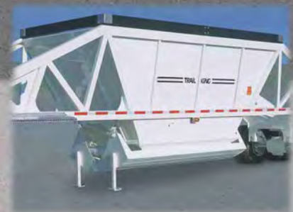
Large 12' Gate and 60" x 106" hopper opening, combined with nearly vertical hopper walls, delivers complete dumping of even the stickiest materials.
