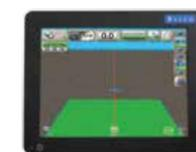
**Field Computer** The Raven™ Viper™ 4 field computer, mounted to the right "A" pillar, is a highly capable controller, delivering the ultimate combination of operating power and program capabilities. With extra hardware, these units can handle multiple system functions, including Raven AccuBoom™ and AutoBoom®.
