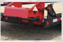
Strong, channel side ladder-style ramps with patented Auto-Latch® ramp hold-ups.
