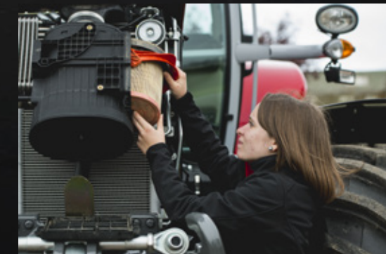
Engine air filter is easy to access and clean.
