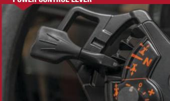
All Global Series tractors come with a clutch control button on the gear shift for simple and clutch pedal –free gear shifting. To change gears in Global Series tractors, press and hold the clutch control button, shift to the desired gear, and let off the clutch control button.
