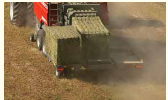
Large bale accumulators collect and group bales in the field.
