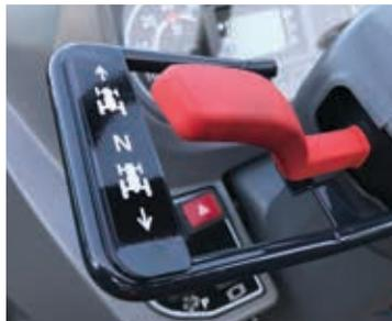
**A handy shuttle-shift lever on the steering column** lets you change direction fast and easy—ideal for loader work.
