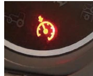
**Cruise control feature is standard** with the hydrostatic transmission and lets you set a precise working speed—just engage and go. Pressing the brake pedal or the forward pedal disengages the system.
