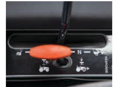
**Get extra traction for tough jobs** and difficult conditions with on-demand four-wheel drive. Just push the lever downward to engage, pull it up to disengage.
