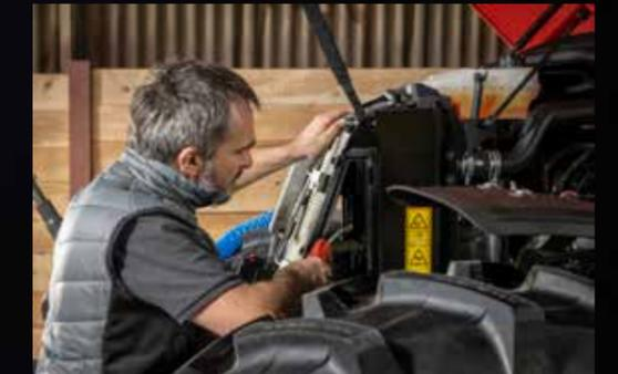
Cooling package is easily accessible to make cleaning faster and easier.
