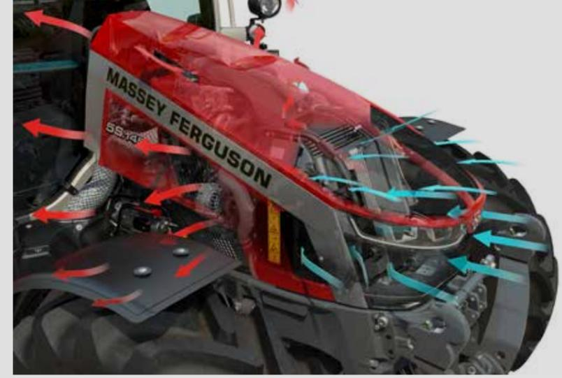
A new optimised airflow system improves engine cooling, which increases performance and boosts efficiency. Thanks to renewed wide grills, all radiators have full access to fresh air (thanks to the new design), providing maximum efficient cooling.
