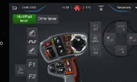
**ISOBUS MultiPad switch assignment.** ISOBUS implements can be controlled directly using the MultiPad lever. Having all controls (tractor and implement) on the same lever is a lot more convenient than using additional displays and levers.
