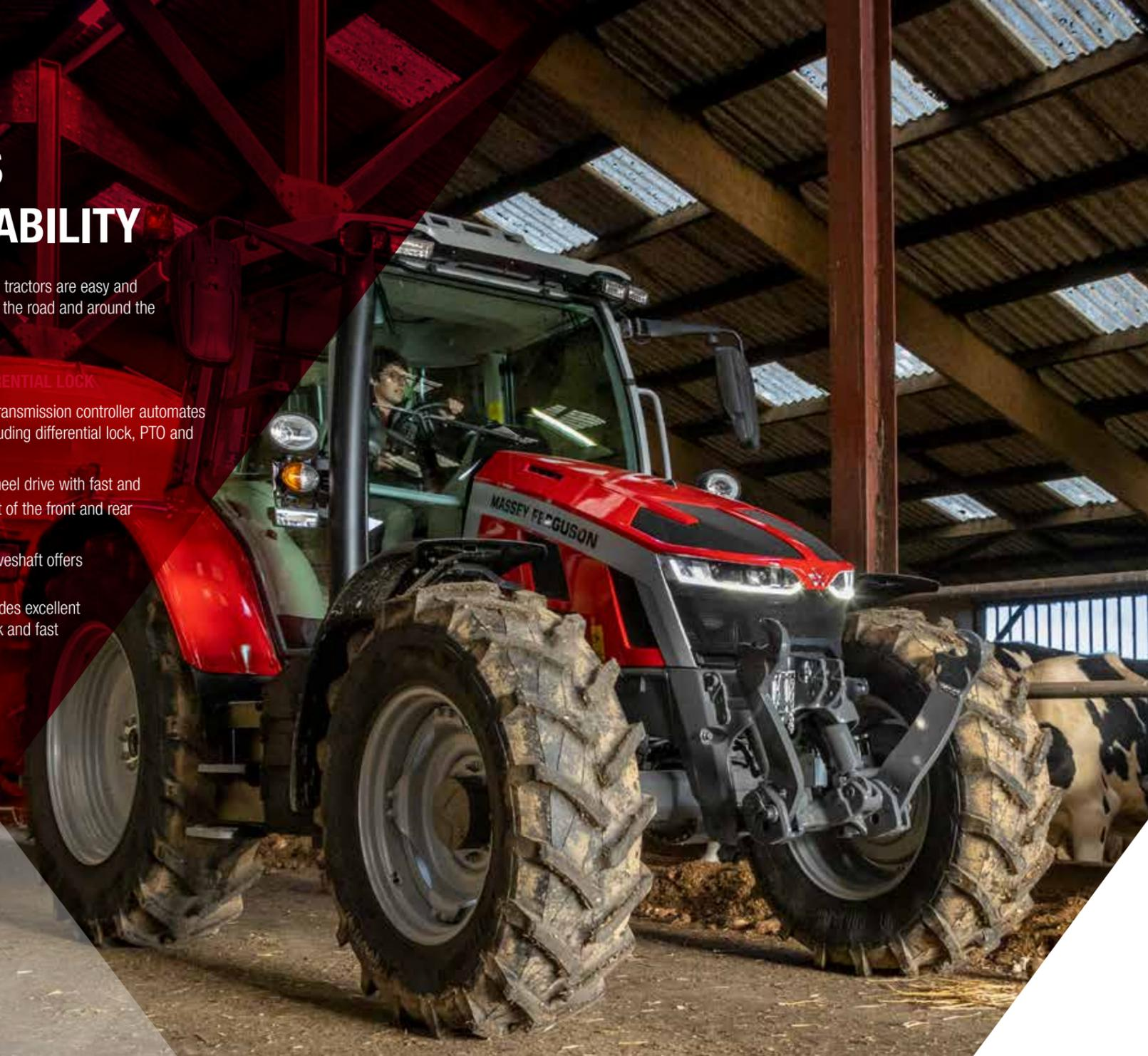
A new, stronger suspended front axle offers an industry-leading 4m turning radius. Working with the new 3t capacity front linkage, which can now lift an extra 500kg, it helps improve efficiency, enabling the tractors to use larger front-mounted equipment. Extra comfort is offered by the electronically-controlled hydraulic suspension, which uses two longer stroke cylinders and three accumulators to absorb shocks.
