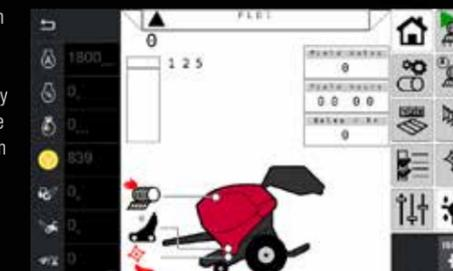
**ISOBUS for total implement control** – ISOBUS allows an implement manufacturer's control system to be displayed on the terminal screen, saving owners and operators time and money, with no need to install additional monitors in the cab. Simply plug the implement lead into the tractor's ISOBUS socket and the system automatically uploads the operating menus and displays on the screen. MF 5S ISOBUS applies to the AEF certification.
