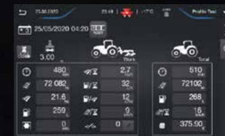
**Memorise data and settings** – Unlimited number of user settings configurations enable the system to record information during operation on area worked, fuel use, hours worked and much more. All the settings and parameters can be stored by the Datatronic terminal. All these settings can be stored and recalled to find the previous setting that was used on a tractor.
