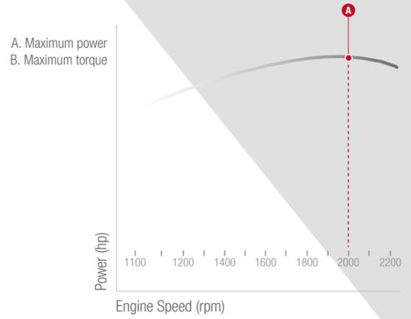
This curve clearly shows how high level of torque is maintained between 1300 and 1900 rpm for greater torque ability and constant PTO Speed.
