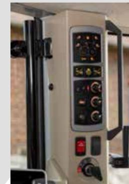
Accurate electronic control provides convenient and simple linkage operation. The ELC potentiometer is carefully positioned to the right of the operator for comfortable and easy use, providing precise control of implement depth as well as lifting and lowering the linkage.
