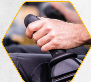
100% pilot controls deliver consistent and responsive flow and pressure to meet your application requirement. Boom swing and auxiliary hydraulics are located on the ergonomic joysticks for ease of operation.
