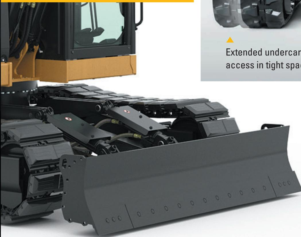
Built for strength and durability, the dozer blade with float functionality as standard assists in back dragging and finish grading. Power Angle Blade options are also available on select models.
