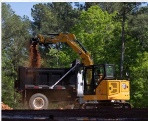
» **Zero tail swing** keeps the upper structure within the width of the tracks to work in the tightest of applications with ease.
