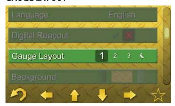
The "Gauge Layout Adjustment" allows the operator to select the Main Monitor Screen display from several available layouts. See "Monitoring Screen." The factory default is Gauge Layout 1. A unique night time scheme is represented by the "moon" icon:
