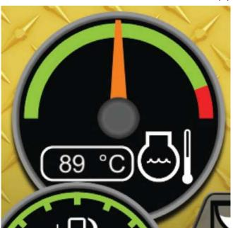
The needle in the red zone indicates that the engine coolant temperature is too high. If the gauge's numerical values are enabled, the background will change from black to red to indicate that the engine coolant is approaching an unsafe temperature. The machine should be stopped soon and the engine set to low idle to allow the engine to cool. See "Display Settings, Digital Readout."
