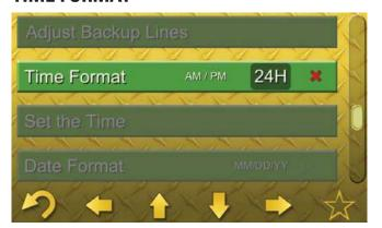
The "Time Format Adjustment" allows the operator to select a 12 hr AM/PM, 24 hr clock format, or disable the clock from appearing.
