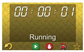
These screens allow the operator to start, stop, and reset a job clock. The job clock saves over the key cycle and starts up automatically on the next startup or operator login. A separate job clock is stored under each operator profile.
