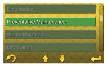
The "Preventative Maintenance" interval screens are pop-up reminders to indicate that a scheduled maintenance interval is approaching. These intervals are based on machine hours and can be reset by the owner after the maintenance is performed. The screens will provide the operator several pieces of information including:
