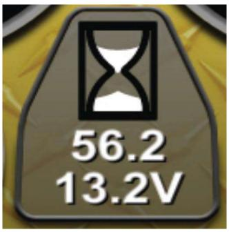
The service hour meter indicates the number of engine running hours for the machine. The hours should be used to determine which maintenance interval service items to perform. The hourglass icon blinks slowly when the engine is running indicating that hours are being accrued. The hour meter also indicates the current battery voltage.
