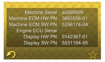
This information can be shared with the Cat dealer to ensure that the machine has the latest software installed to take advantage of any improvements developed since the machine was manufactured.
