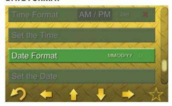
The "Date Format Adjustment" allows the operator to select between three date formats; MM/DD/YY, DD/MM/YY, or YY/MM/DD.
