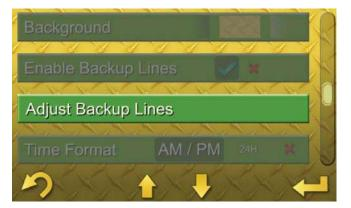
If the Backup Lines are enabled, the "Adjust Backup Lines Adjustment" screen provides the user various adjustments for the Machine Width reference lines and the Rear Distance reference marks.
