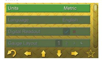
The "Units Adjustment" allows the operator to switch between Metric and English units. The factory default is English.
