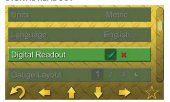
The "Digital Readout" allows the operator to either have the numerical gauge values display turned ON or OFF. The factory default is "ON."
