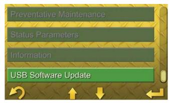
The "USB Software Update" screen allows for the Cat dealer to service the Advanced Display's software as needed.
