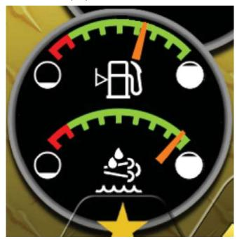
The fuel level gauge indicates the amount of fuel that remains in the fuel tank. The needle in the red range indicates low fuel.
